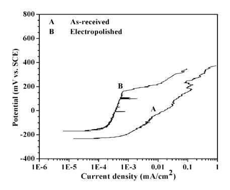
Fig1. Potentiodynamic polarization results for electropolished (red) and as-received (black) in 0.5M NaCl solution and 60mV/min scanning rate<sup>1</sup>
