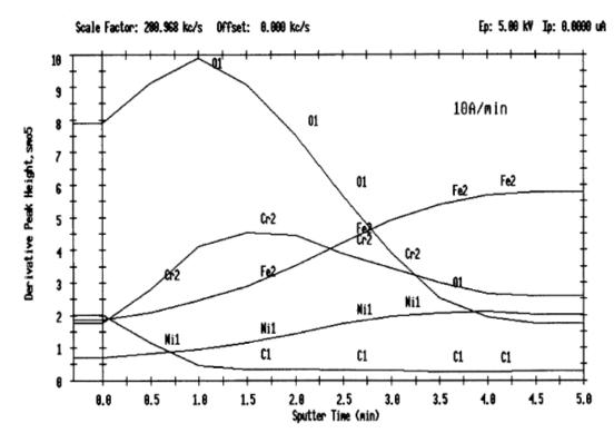
Fig3. Results of AES depth profile analyses, the oxide thickness is 25Å.<sup>4</sup>
