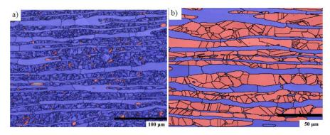
Fig6. EBSD phase map of a) mechanically polished sample and b) electropolished sample (blue=bcc, red=fcc)<sup>9</sup>.
